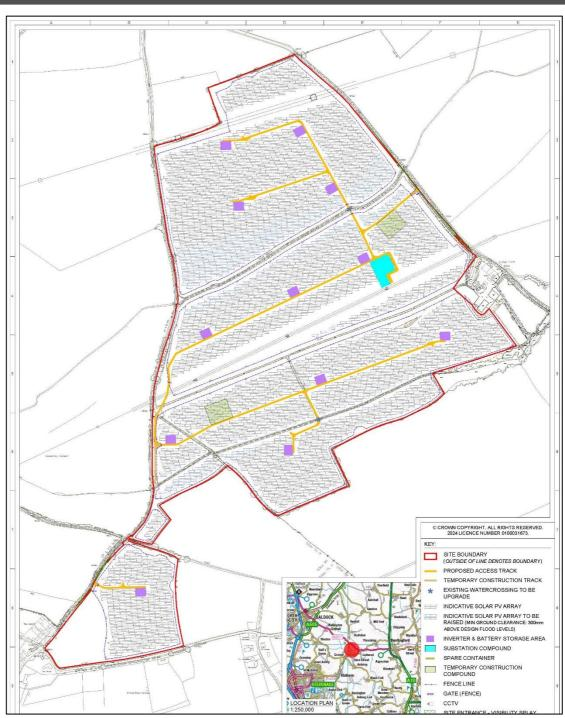
Figure 1 Proposed solar array boundary
