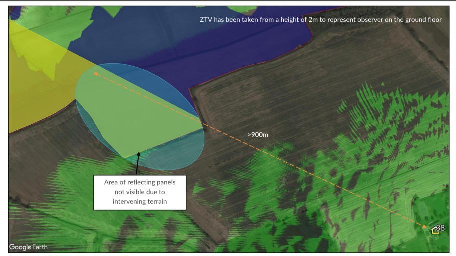
Figure 25 Screening relevant to dwelling receptor 38, including terrain mapping from receptor 38
