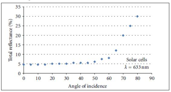
Total reflectance % when compared to angle of incidence
