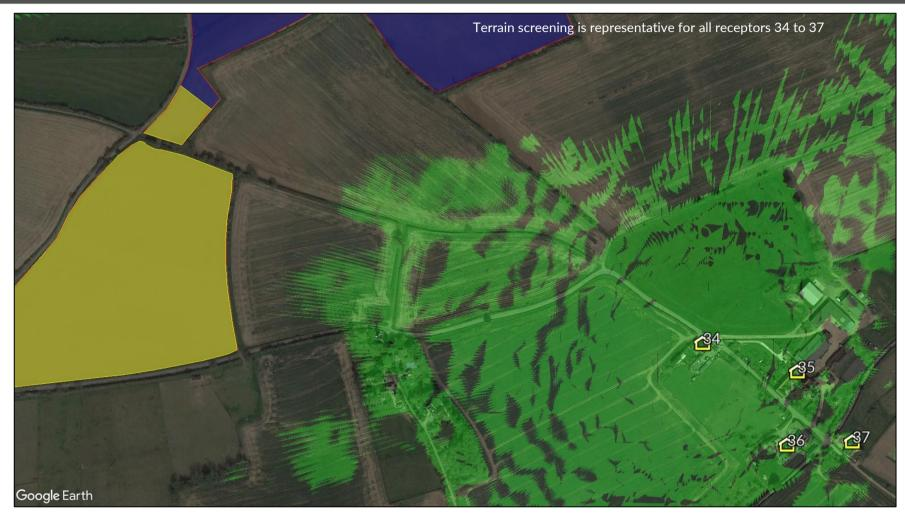
Figure 24 Screening relevant to dwelling receptors 34 to 37, including terrain mapping from receptor 34
