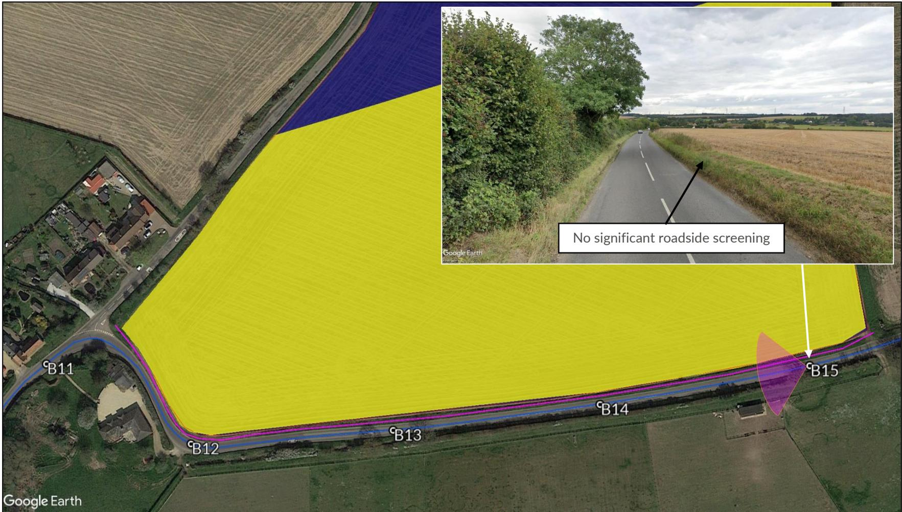
Figure 29 Reflective panel area and proposed screening for road receptors B11 to B15
