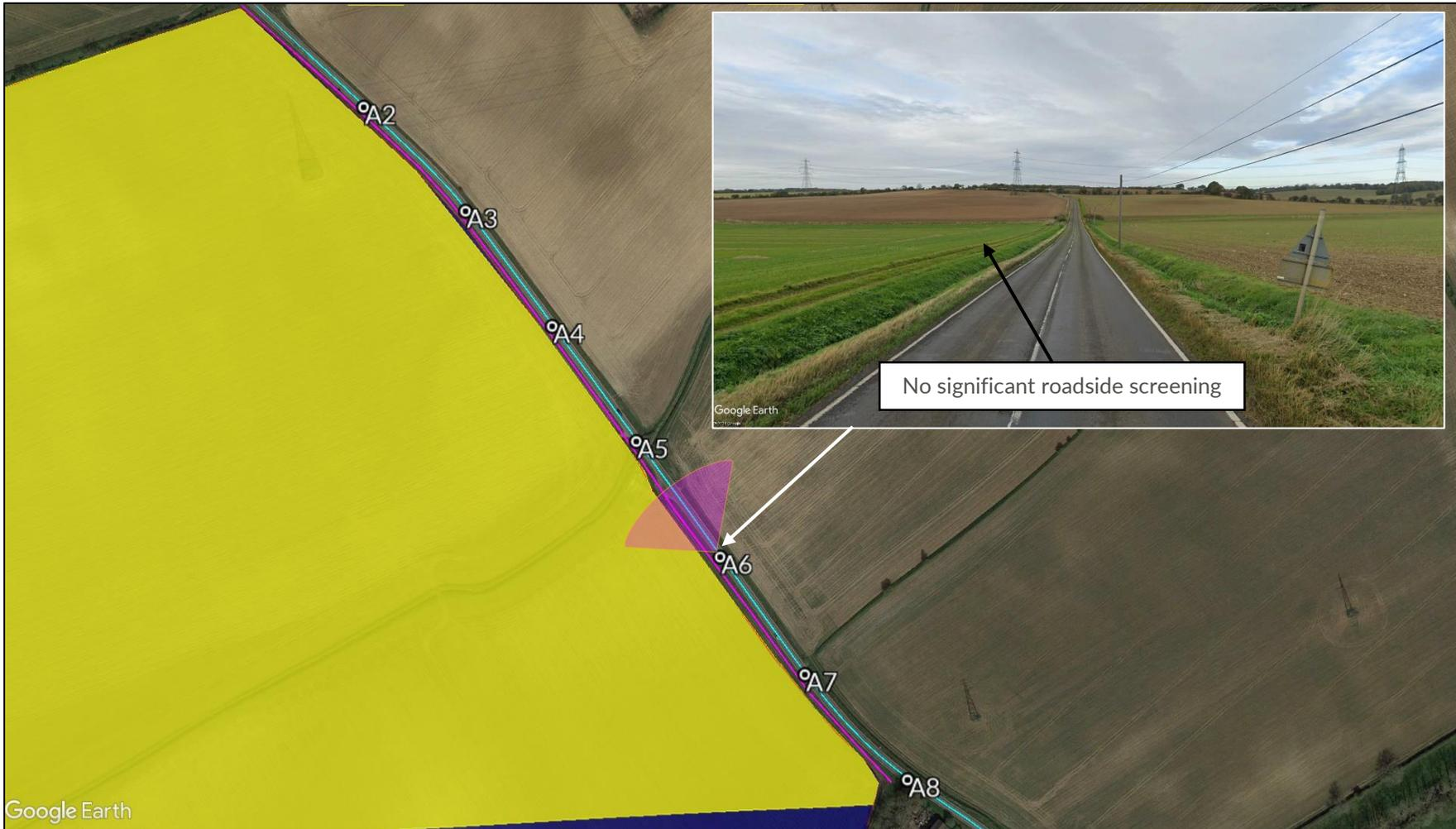
Figure 28 Reflective panel area and proposed screening for road receptors A2 to A8
